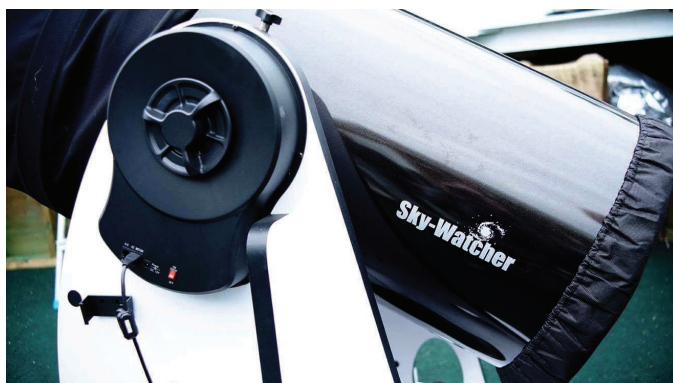
Figure 2 — The larger Sky-Watcher dobs have adjustable bearings on both axes.
